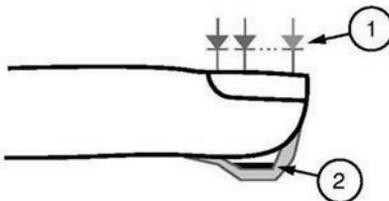
Once Radical-7 receives the signal from the sensor, it utilizes proprietary algorithms to calculate the patient's functional oxygen saturation ( $SpO_2$  [%]), blood levels of carboxyhemoglobin saturation ( $SpCO$  [%]), methemoglobin saturation ( $SpMet$  [%]), total hemoglobin concentration ( $SpHb$  [g/dL]) and pulse rate (PR). The  $SpCO$ ,  $SpMet$  and  $SpHb$  measurements rely on a multi-wavelength calibration equation to quantify the percentage of
