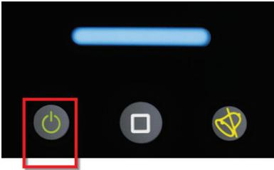
Use the *Power Button* to Power On, put the Radical-7 in Standby Mode, or completely Power Off.
