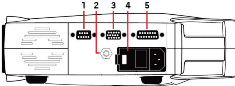
**1. Serial Output connector** - Provides connection with a serial device, including a serial printer, a monitoring system, or PC to the Radical-7. The data is provided in standard RS-232C format. All external device connections to the Serial Output connector must be IEC-60950 compliant.
