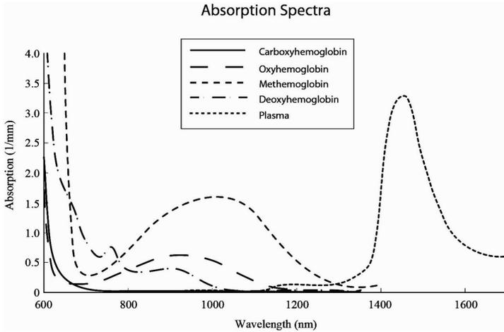
The Radical-7 uses a multi-wavelength sensor to distinguish between oxygenated blood, deoxygenated blood, blood with carbon monoxide, oxidized blood and blood plasma.
