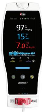
The Handheld contains the majority of the device features. All measurements and device status data are displayed on the touchscreen. All user input is performed through the touchscreen and control buttons. The sensor cable connector is located on the Handheld.
